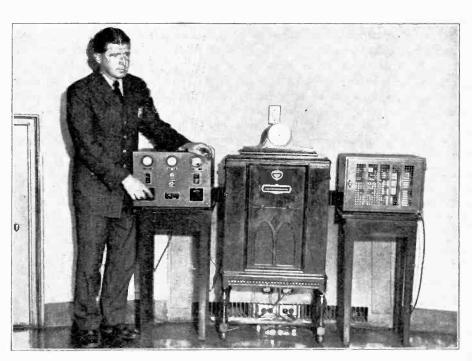
Dispatcher Carl Vollmer shown at the frequency monitor which checks wave lengths. This is a part of the New York police radio equipment
